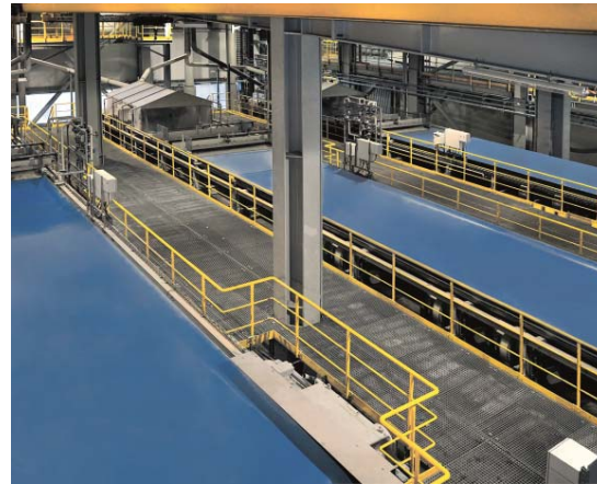
Picture 2: With VACUBELT® filter belts for continuously operating vacuum belt filters, GKD offers high-performance process belts with consistently high dewatering performance and robust lateral stability.
